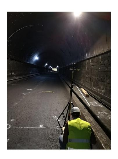
6 x 6 = 36 points on crosssection measured 140 m away from jet fan, in accordance with BS EN ISO 5802: 2008+A1:2015
