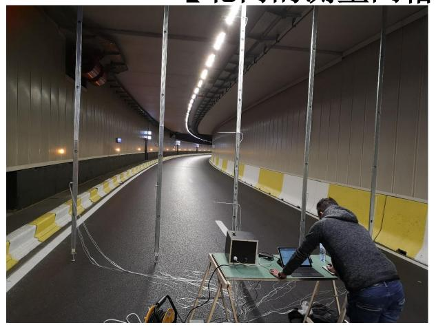
5 x 5 = 25 points on cross-section measured near the north portal, in accordance with BS EN ISO 5802: 2008+A1:2015
