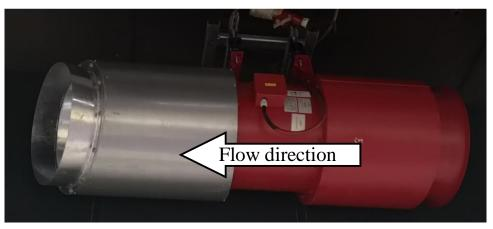
Experimental comparison between unidirectional jet fans (3 conventional jet fans and 3 MoJets) undertaken; 100% additional thrust with MoJet measured by ULB University. 【进行了单向射流风机(3个常规射流风机和3个 MoJets风机)之间的实验比较; ULB大学测出的 MoJet 的推力增加100%。】
